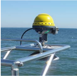
Figure 1 WaveRadar REX on Swanage Pier
