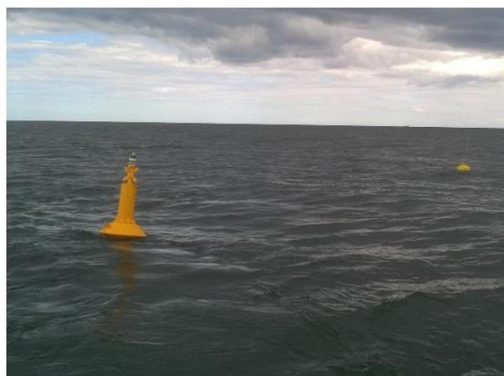
The seabed moorings at Whitby consist of a Datawell shallow water mooring with a single 30 m rubber cord, 1.2 m diameter yellow marker buoy complete with radar reflector, St. Andrew's cross and navigation light (GpFl Y 5/20) and riser line comprising 16 mm diameter combined wire and rope. A similar marker buoy may be installed at the Scarborough site should the Whitby Marker prove successful.
