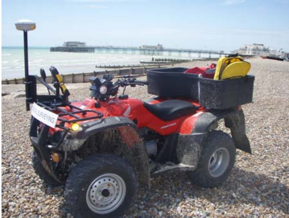
Figure 1 RTK GPS equipment mounted on ATV
